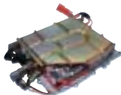
DC-DC converter for the Prius
