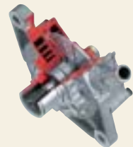
Viscous-Type Power Heater (Vehicle Cabin Supplementary Heater)
