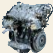
1CD Diesel Engine (Displacement: 2.0 Liters, Used in the RAV4 for Europe and Corolla)
