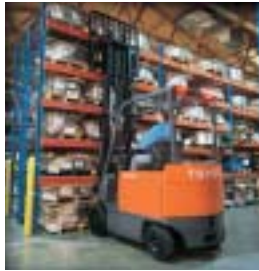
7FBCU35 Electric 4-Wheel Cushion Tire Counterbalanced Forklift Truck
