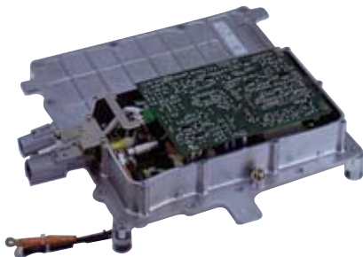
DC-DC Converter for the Prius
