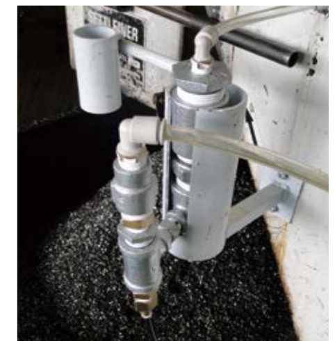
Iwama Loom Works' karakuri pump evolved to eliminate parts processing
