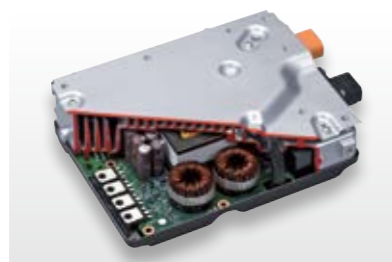
DC-AC inverter mounted in the new Prius
