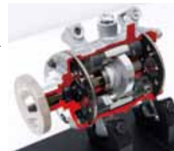
10SA13 fixed-displacement type compressor produced by TACI and installed in TMC's IMV series vehicles and the Etios
