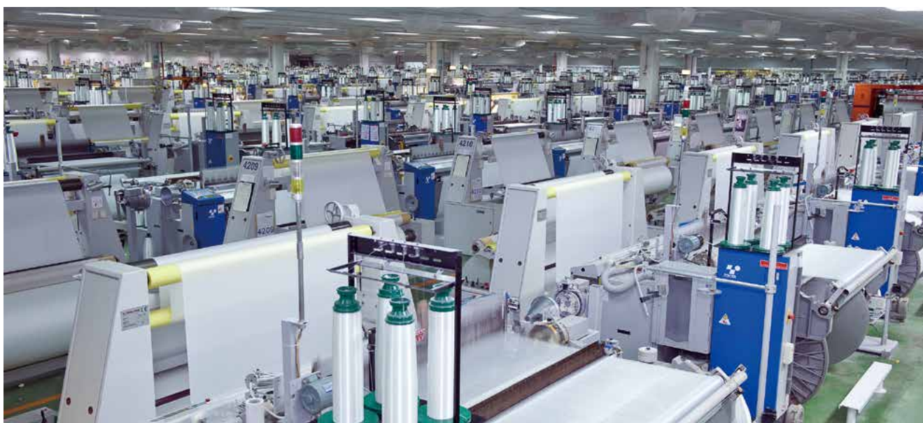
JAT710 air-jet looms in operation at Nan Ya Plastics
