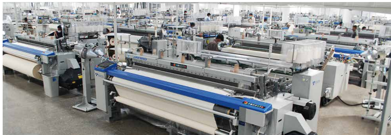
JAT810 air-jet looms in operation at Nishat Mills, Ltd
