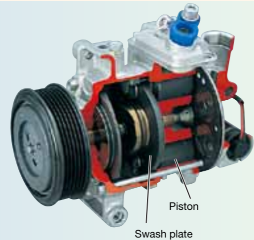
By changing the angle of the swash plate to adjust the piston stroke, the compressor automatically controls the cooling capability.
