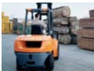
7FG/D35 Internal combustion counterbalanced lift truck (3.5-5 ton)
