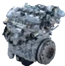
2AD diesel engine (Displacement: 2.2 liters, used in the Avensis, RAV4, Corolla Verso and Lexus IS)
