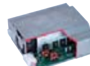
DC-AC inverter for the Tacoma (400W)
