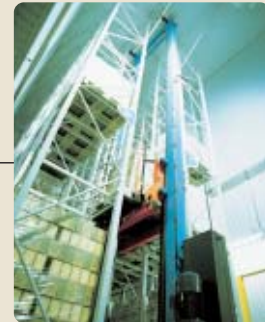
Automated storage and retrieval systems
