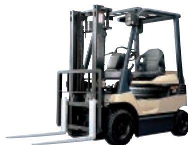
GENEO-B (7FB): An electric-powered forklift equipped with a dedicated AC drive system for forklifts as standard equipment. With high basic performance and operability, the GENEO-B shows the way forward for electric-powered forklifts.
