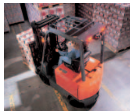
7FBCU25 Electric cushion tire counterbalanced lift truck
