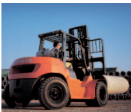
7FGU70 Internal combustion pneumatic tire counterbalanced lift truck
