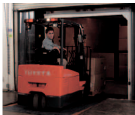
7FBEU20 Three-wheel electric counterbalanced lift truck
