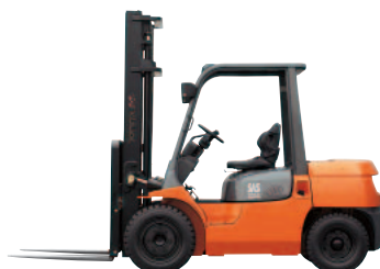
Toyota 7FG/D40 Internal combustion counterbalanced lift truck (3.5-5 ton)
