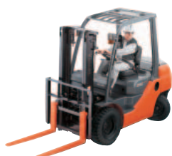
GENEO (8FG25) Internal combustion counterbalanced lift truck
