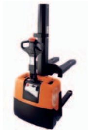
BT Minimover Powered stacker truck
