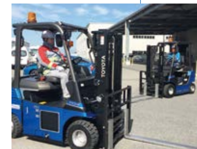
Feasibility test of FC lift truck
