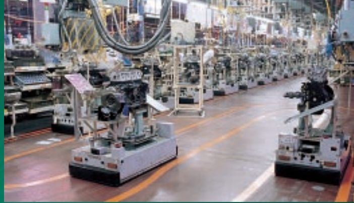
Engine assembly line using automatic guided vehicle systems
