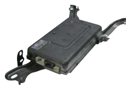
DC-DC converter for the new Lexus RX Hybrid
