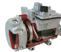
ES27 electric compressor (Scroll type)
