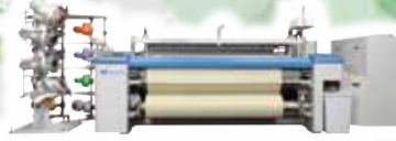
Air-Jet Loom Inserts weft yarn using air and enables weaving of textiles with various textures
