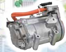
Electric Compressor Fitted in hybrid vehicles (HVs) and enables use of air conditioner even during idling stop
