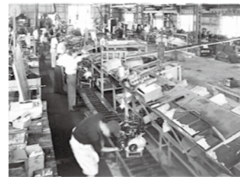
S-type gasoline engine assembly line
