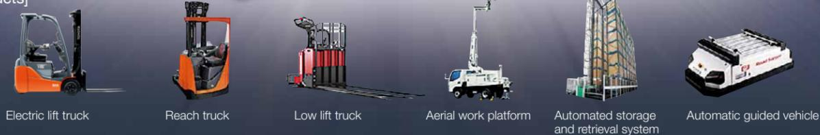
The Materials Handling Equipment Segment develops, produces, sells and provides services for a broad range of products, from industrial vehicles centered around a full lineup of lift trucks (0.5- to 43-ton capacities) to materials handling systems.
