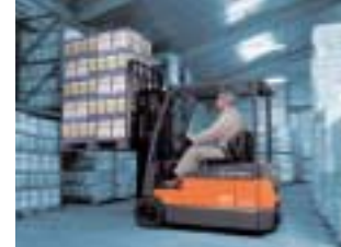
7FBEF15 Three-wheel electric counterbalanced lift truck (48V)
