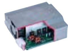
DC-AC inverter for the Tacoma (400 W)
