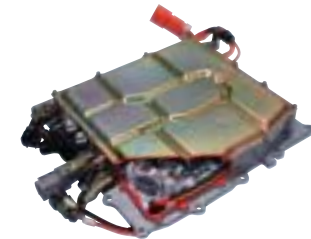
DC-DC converter for the Prius
