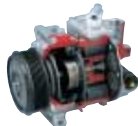
7SEU17 compressor (Externally controlled, clutchless type)
