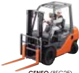
GENEO (8FG25) Internal combustion counterbalanced lift truck
