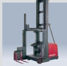
Raymond Swing-Reach Truck Very narrow aisle truck
