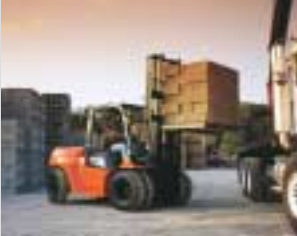
7FGU70 Internal combustion pneumatic tire counterbalanced lift truck
