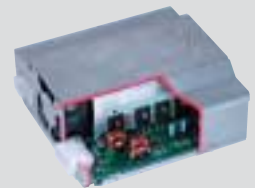
DC-AC inverter for the Tacoma (400W)
