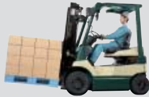
GENEO-B (7FB15) Electric counterbalanced lift truck
