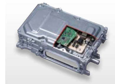
DC-DC converter mounted in the new Prius
