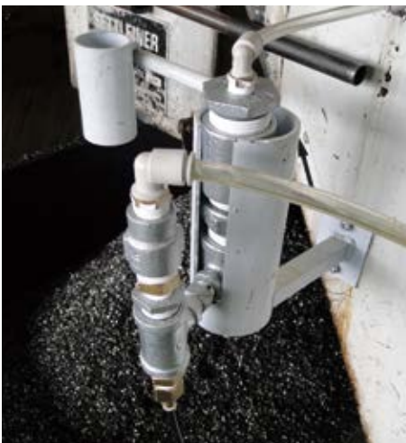
Iwama Loom Works' karakuri pump evolved to eliminate parts processing
