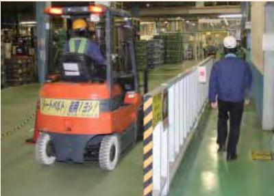
Separating walking and lift truck operating zones (Kariya Plant)
