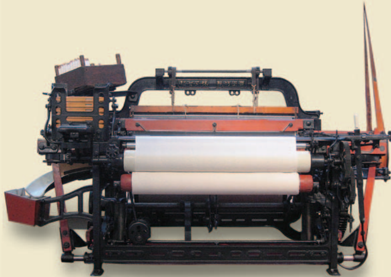
In August 2007, the first model of the non-stop shuttle-change Toyoda automatic loom, Type G, was certified as a Mechanical Engineering Heritage asset.
