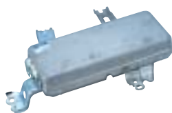
DC-DC converter for electric power steering for the Harrier Hybrid (RX 400h) and Kluger Hybrid (Highlander Hybrid)
