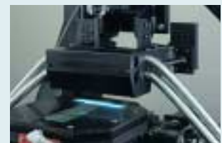
Circuit board inspection system with high-resolution line scan camera
