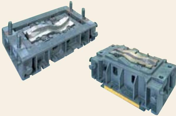
The Machinery & Tools Sub-Division designs and manufactures high-precision, high-quality automobile press dies for TMC. We will continue to contribute to TMC's business with press dies that offer excellent quality, cost efficiency and fast delivery times.
