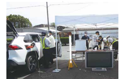
Disaster prevention drill using AC inverter's power source functionality
