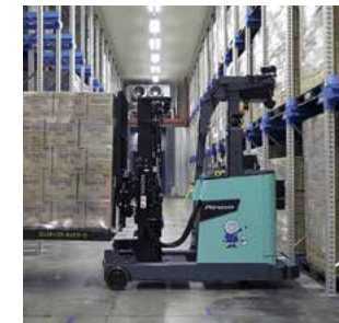
Automated lift truck operating in a freezer warehouse
