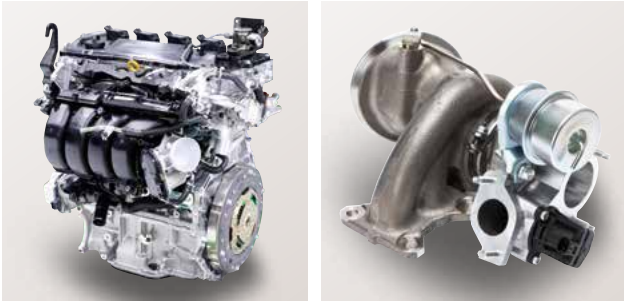
2.5-liter A25A engine for HEVs
