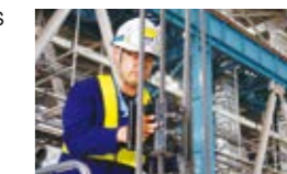
Checking the internal breaking of wire ropes
