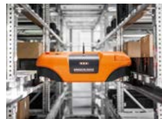
Shuttle-type automated storage and retrieval system
