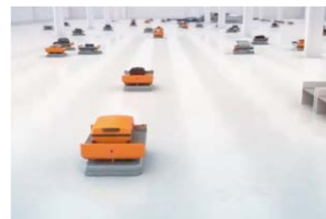
Baggage handling system utilizing autonomous vehicle technology for airports
