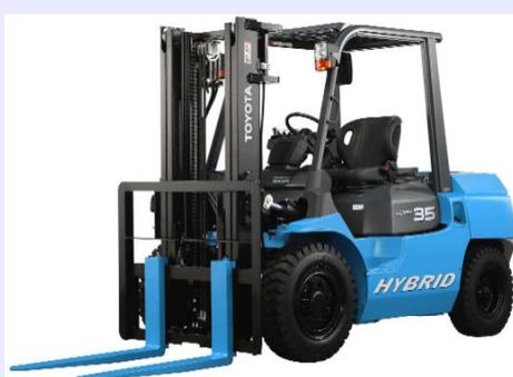
Internal-combustion hybrid lift truck
