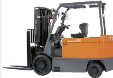
Large electric lift truck (5.5- to 8.5-ton)
