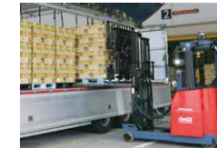
4-fork autonomous lift truck for truck loading and unloading
