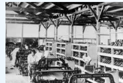
Production of Type G automatic looms
