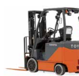
Cushion tire lift truck (produced in North America)
