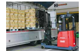
4-fork autonomous lift truck for truck loading and unloading
