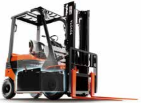
geneB electric lift truck equipped with a lithium-ion battery
