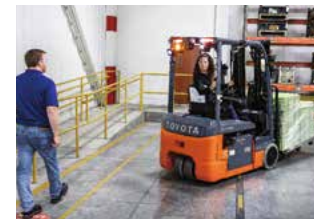
Three-wheel electric lift truck to which operator assist and other functions have been added
