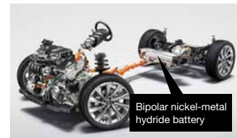
TMC's dual boost hybrid system
