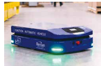
Bastian's mini load autonomous vehicle (autonomous mobile robot) developed in-house
