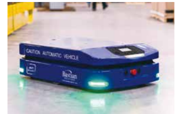
Bastian's mini load autonomous vehicle (autonomous mobile robot) developed in-house
