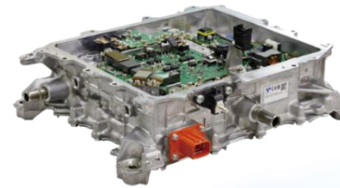
Unit Integrating an On-Board Charger and DC-DC Converter
