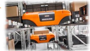
Shuttle type Automatic warehouse
