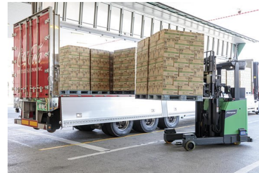
Autonomous lift trucks for truck loading and unloading (4-fork type)
