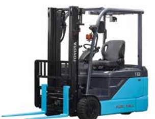
Fuel cell lift truck
