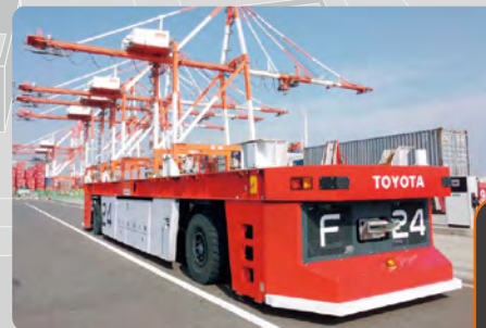
Container transport AGV system
