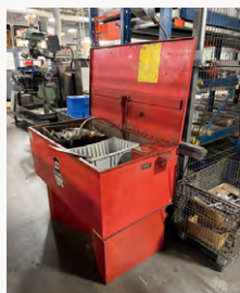
Removed Parts-Cleaning Machine
