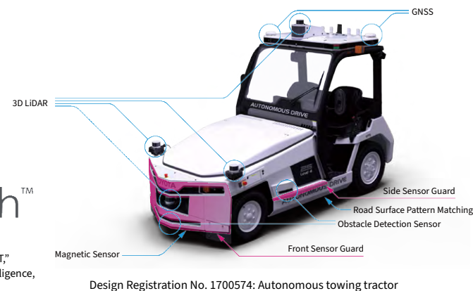
Design Registration No. 1700574: Autonomous towing tractor
