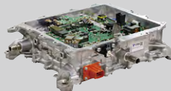
Integrated on-board charger and DC-DC converter unit
