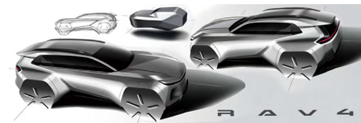
The polygon theme in the exterior design was maintained but we looked to incorporate a new proportion that expands cargo space
