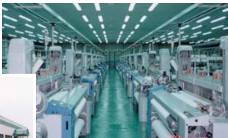
JAT610's up and running on the mill floor
